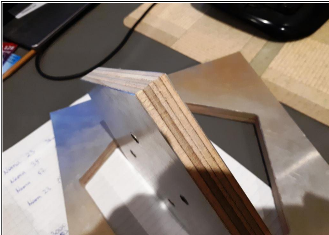
An aluminium and ply laminate test cut.
