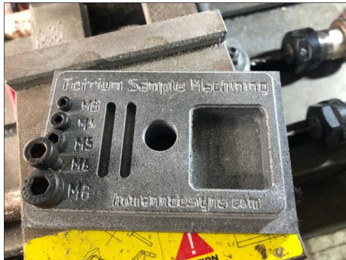
Tetrium-S can be threaded. For best strength a screw diameter to depth ratio is 1:2 ie a 6mm screw would require a 12mm deep thread. If the thread is to be highly loaded then a suitable threadlocker adhesive should be used.
